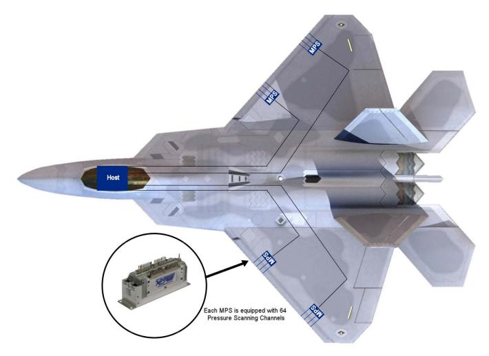
The MPS4264 is an intelligent 64 channel pressure measurement device. This device is a stand-alone scanner and handles all of the A/D conversion at the module level. Communication to the module is Ethernet TCP/IP or UDP. A TCU (Thermal Control Unit) is available to help stabilize sensor temperature in extreme conditions.
