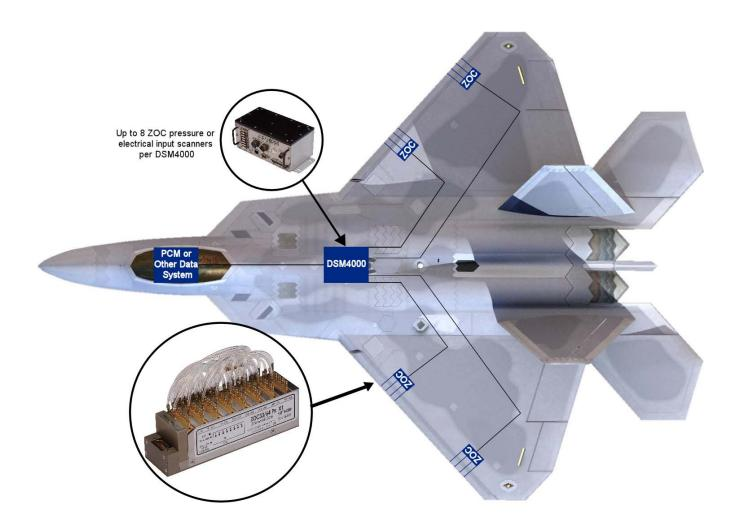
The DSM4000 Digital Service Module is designed to be used with Scanivalve ZOC pressure and electrical input scanners. The DSM4000 contains 8, 16 bit A/D's with each A/D supporting one ZOC module. Communication is enabled via Ethernet or optional ARINC429. Data is output in temperature corrected engineering units.
